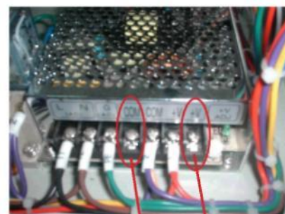
DC power output terminal DCC24V
